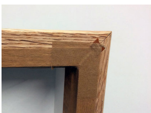
Step 9: Place a brown tape over the complete length of each frame length (4 sides), cut-in the corners and fold inside direction of the frame to fix the folded angles of the Media.
